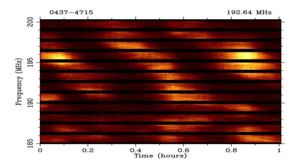
Figure 1: Dynamic spectrum of pulse intensity from MWA observations of the timing-array millisecond pulsar J0437-4715 (Bhat et al. 2016). The modulations and patterns seen in pulse intensity arise from multipath propagation of pulsar signals through the intervening interstellar medium (ISM). The MWA's 80-300 MHz operating frequency range is well suited for detailed characterisations of such propagation phenomena in the ISM toward all Parkes timing-array pulsars.
