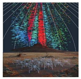
The effect of the ionosphere on the sources seen by the MWA during a particularly extreme event. Each arrow represents the shift in position of a source; colours indicate directions. Earth's magnetic field lines are shown as white lines.
