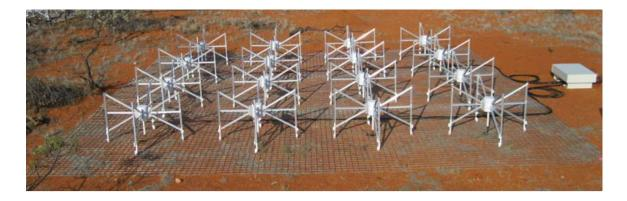
Figure 1: An MWA antenna 'tile'
