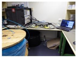
Figure 1: Laboratory measurements of RFoF links.
