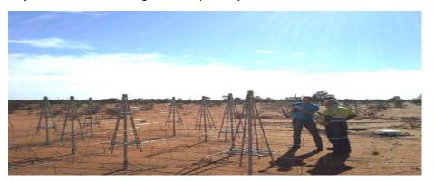
Figure 1: SKA\_Low antennas installed at the MRO for trial purposes.
