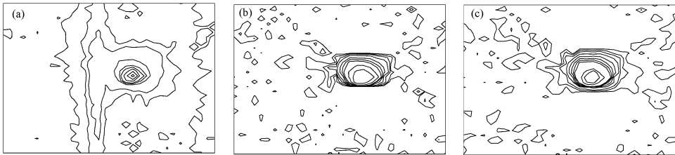
图 10 星像的等高图. (a) 原始星像, (b) TopHat 方法处理结果, (c) Spread TopHat 方法处理结果 Fig.10 Contour plot of images. (a) Original image, (b) Transformed by TopHat. (c) Transformed by Spread TopHat
